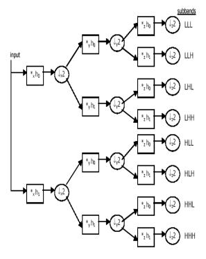
Fig. 5 Block diagram of a single level decomposition for the 3D DWT
